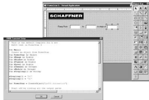
The Test Development Kit (TDK) is a built-in test environment for PowerStar 5's ATE control and test development software, providing a powerful means for creating custom data driven tests within PowerStar 5.
